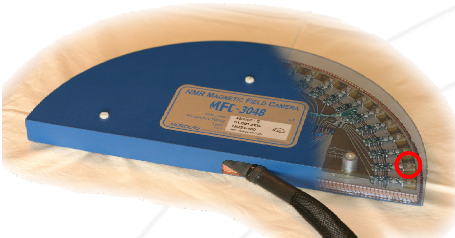
Figure 11. Close-up of an NMR probe array. Each probe – one of them is circled – is mounted on its own circuit card. Such probe arrays typically contains 24 or 32 probes (maximum 96).
